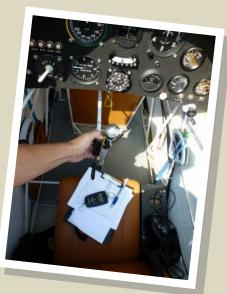
Many tests were undertaken to improve the engine oil temperature behavior. Often it did run a little cold whereas on some occasions it got close to its limit. A radiator system combined with a new thermostat valve showed obvious improvement and will be available as an option in future.
